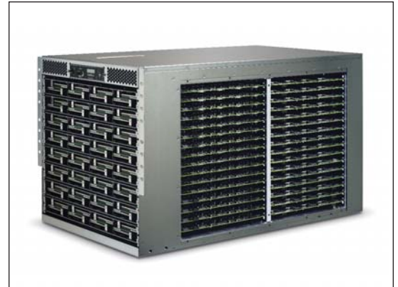
SeaMicro SM10000 without covers illustrates its compact design.
